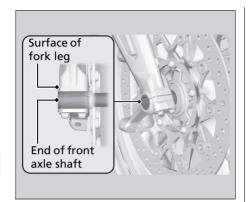
5. Install and tighten the axle bolt.
