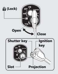
The shutter will automatically close when you remove the ignition key at the (Lock) position.
