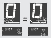
2 Press the MODE button. The speed and mileage unit is set, and then the display moves to the changing of the temperature gauge unit.
