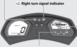
Neutral indicator Comes on when the transmission is in Neutral. ABS (Anti-lock Brake System) indicator
