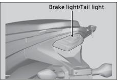
The brake and tail light uses several LEDs. If there is a LED which is not turned on, see your dealer for servicing.
