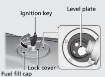
Do not fill with fuel above the level plate. Fuel type: Unleaded gasoline only Recommended fuel octane number: Pump Octane Number (PON) 86 or higher. **Tank capacity:** 4.62 US gal (17.5 liters)
