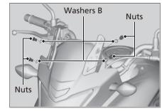
**4.** Set the all nuts and the washers B to the low position holes or high position holes.
