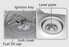
Do not fill with fuel above the level plate. **Fuel type:** Unleaded gasoline only Recommended fuel octane number: Pump Octane Number (PON) 86 or higher. **Tank capacity:** 4.57 US gal (17.3 liters)
