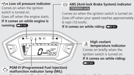
Comes on briefly when the ignition switch is turned on with the engine stop switch in the  $\bigcap$  (Run) position. Comes on when the ignition switch is turned on with the engine stop switch in the  $\bigotimes$  (Off) position.
