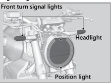
The headlight, position light and front turn signal lights use several LEDs.
