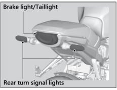
The brake light, taillight and rear turn signal lights use several LEDs.
