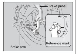
When the brake is applied, an arrow attached to the brake arm moves toward a reference mark on the brake panel. If the arrow aligns with the reference mark on full application of the brake, the brake shoes must be replaced. See your dealer for this service.
