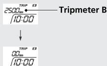
Also, the tripmeter A, average fuel mileage, and fuel consumption will automatically reset by refuelling more than the reserve amount and riding your motorcycle for 0.1 km (0.06 mile)
